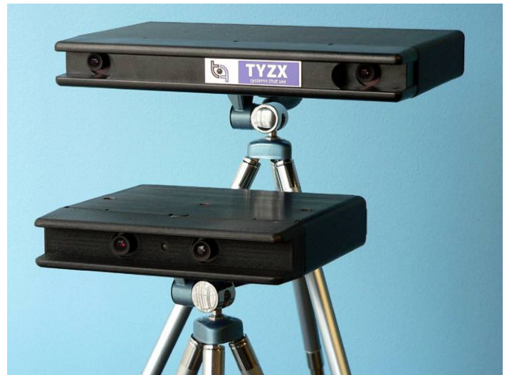
The DeepSea G2 Vision System is a self-contained, intelligent, real-time 3D sensor designed for production deployment of 3D applications in security, robotics and interactive systems
