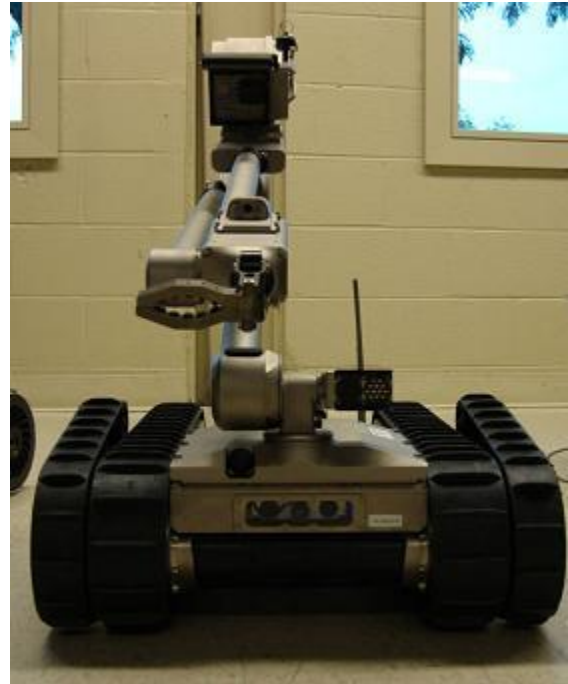
An iRobot PackBot configured with a TYZX G2 Vision System in its payload for situational awareness and obstacle detection/obstacle avoidance.
