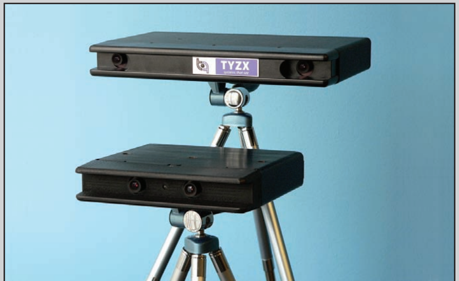
Figure 2. Cameras range from narrow (3-cm) baselines that can be used to study items only 15 to 20 cm from the camera to very long-baseline (up to 33-cm) specialty cameras that can be used to look at objects hundreds of yards away. The baselines on the cameras shown are 6 cm and 22 cm.
